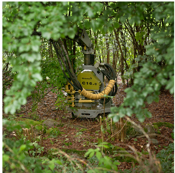
Bracke C16.c, accumulating felling head for silviculture and biomass applications.
